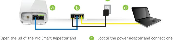
fastened to the POE port. Locate the PoE Adapter and connect the 30 ft PoE cable to the REPEATER port on the PoE
