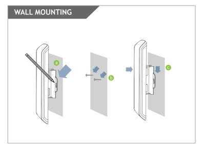
and mark two pilot locations through the mounting hole on the wall. Remove the SR600EX and securely drill two screws
